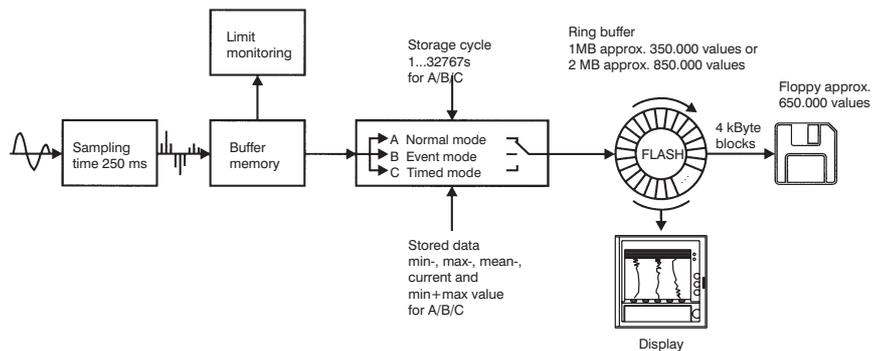
The Engineering Tool (see Accessories) provides the function „Storage period“, with which the recording period is computed for the selected configuration.
