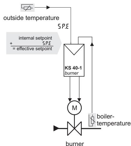
*Application example for synchronisation control with additional master controller:*
