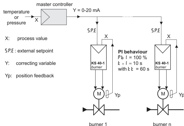
*Application example for synchronisation control for two burners:*
