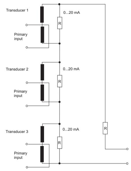
The resistors must be matched in such way that the resulting output signal can be read by the analogue input board from the PLC.
